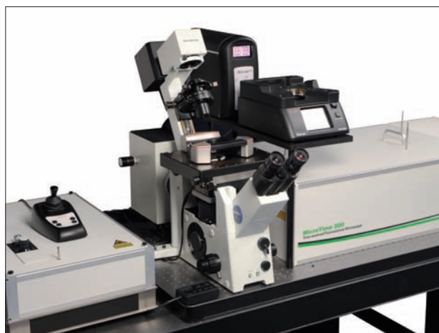
Fig. 1: Combined setup of the MicroTime 200 and the BioScope Catalyst. The AFM with its sample stage is mounted on the inverted microscope body of the MicroTime 200. The MicroTime 200 is configured for objective scanning.
